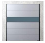
Aluminium panel with a clear acrylic glass without glazing bars – VISUAL. The panel is painted on both sides in the external door colour. Available with MakroPro 2.0 doors So  $\leq$  4,000 [mm] and Ho  $\leq$  4,000 [mm] with glazing units: No-Scratch, "R", Satin, and Grey for So  $\leq$  3,000 [mm].
